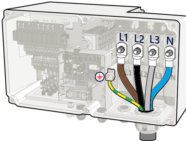
Figure 24: Connecting wires to the AC terminals
