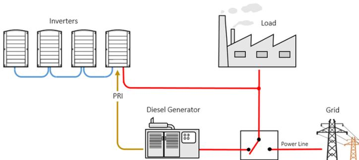
Figure 35: Example of Alternative Power Source System
