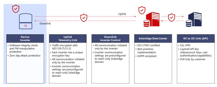
SolarEdge inverters have multiple security layers – including both built-in and third-party mechanisms – that are designed to limit exposure to opportunistic and targeted cyber-attacks.
